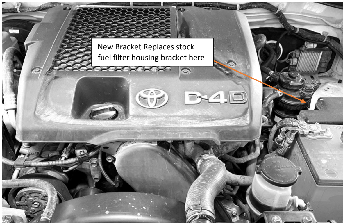
N70 Hilux Engine Bay Overall View
