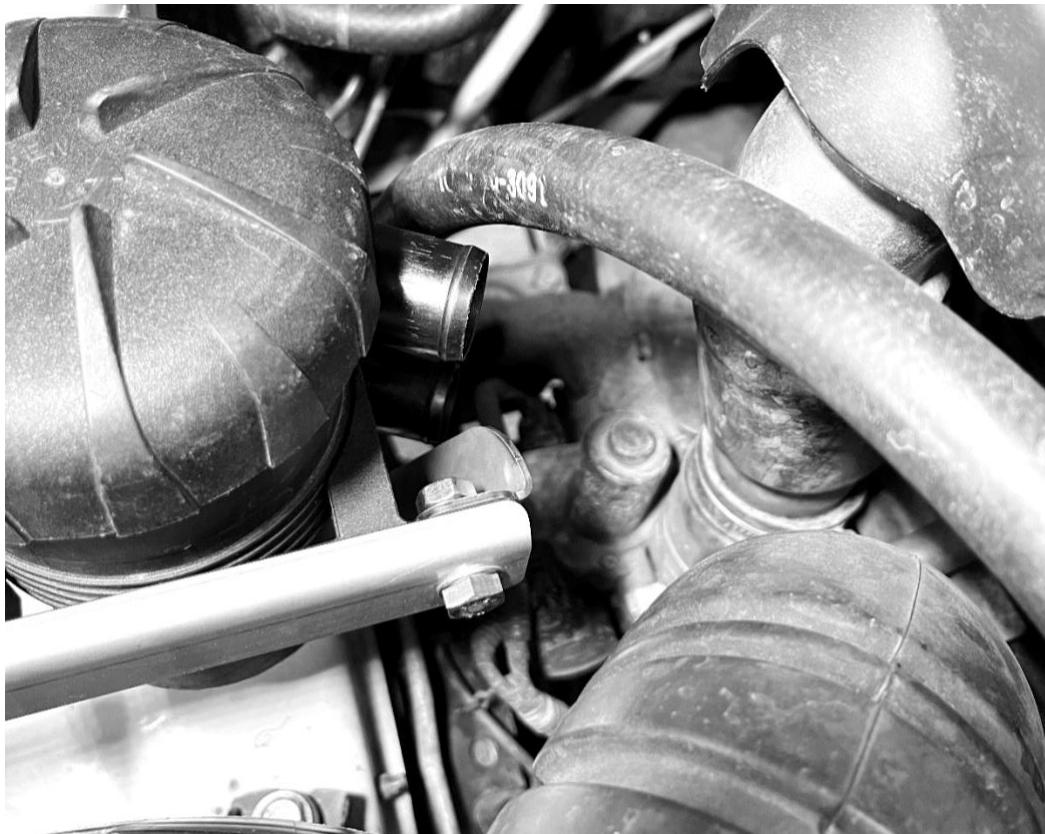
ProVent 200 bolted to bracket– Please note ProVent rotation in this image is correct, refer to the image on the last page of this installation guide for how to rotate the unit. Brace upper mounting location shown.
