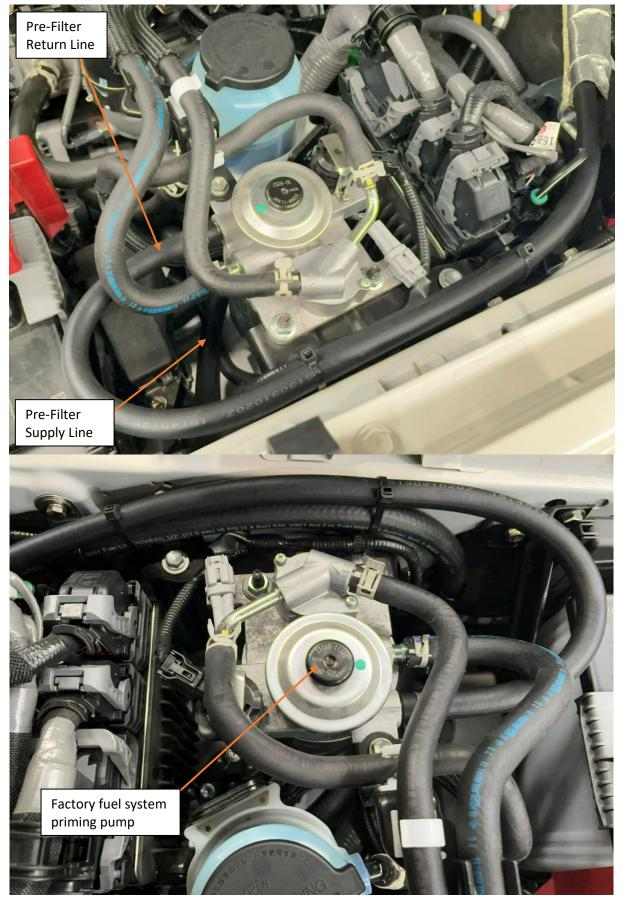
LC70 2.8L factory fuel system priming pump
