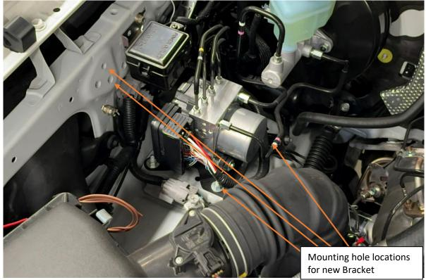
Image shows new bracket mounting location.
