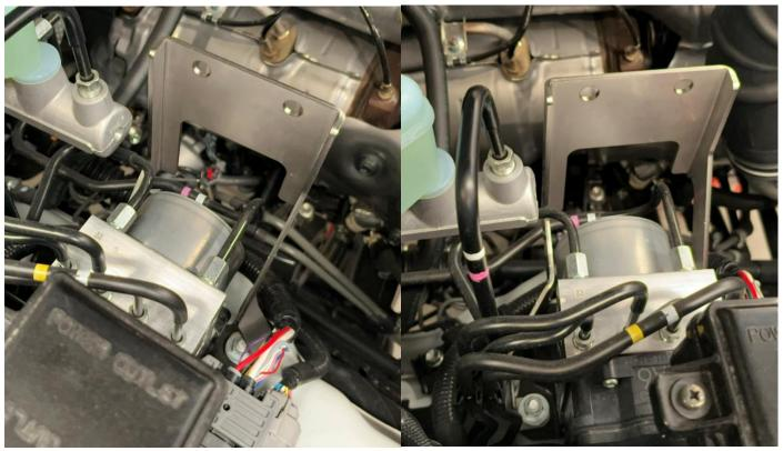
Mounting Bracket A fitted to the vehicle.
