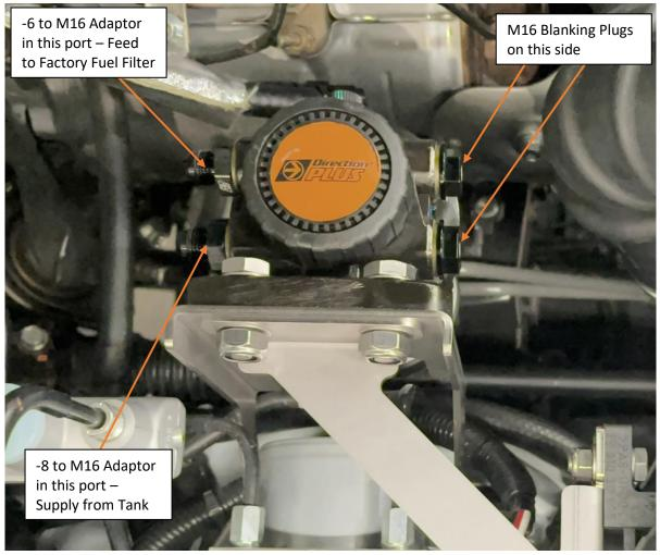
FM100 in place on bracket with Adaptors installed.
